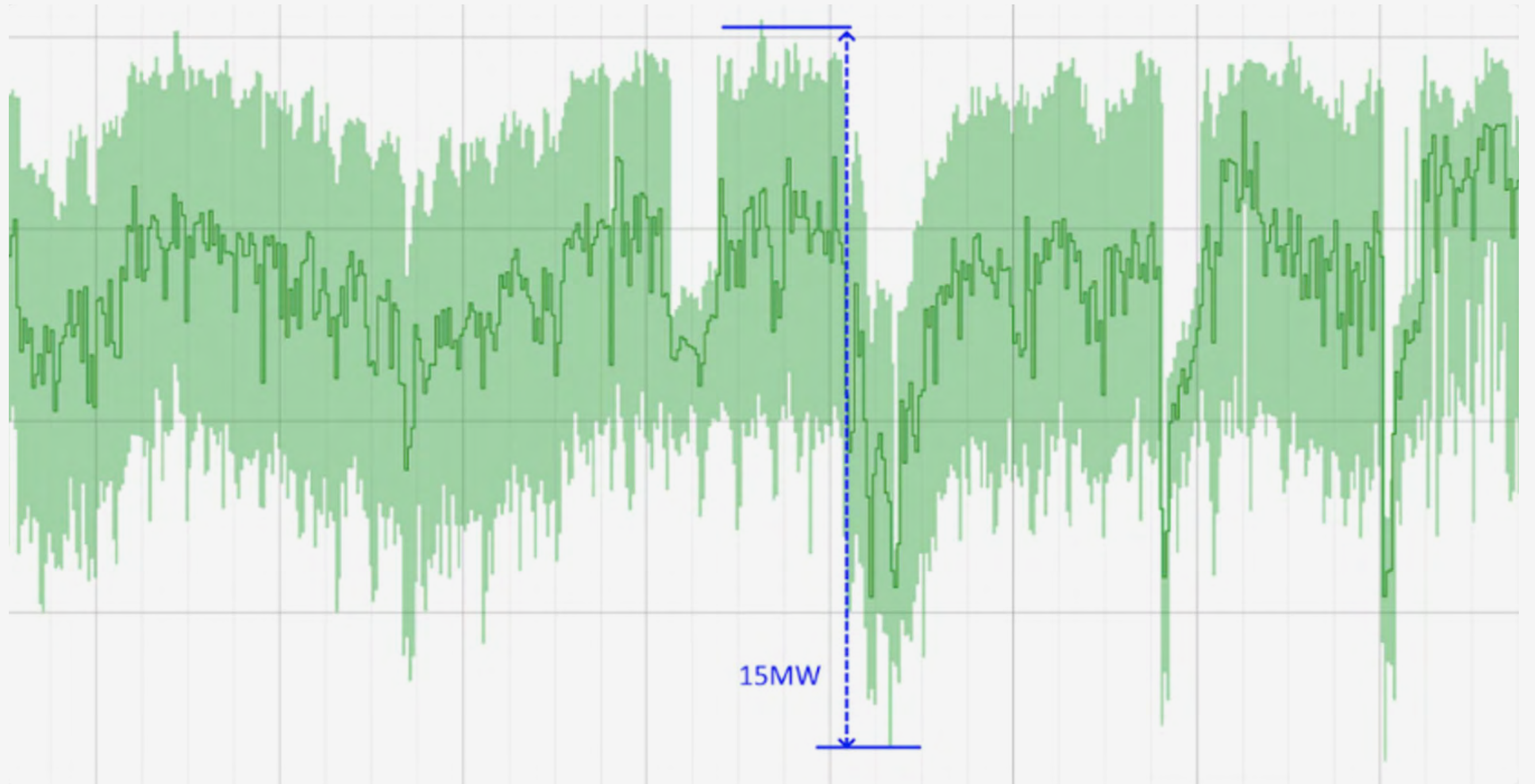
Fig. 1. Large power fluctuations observed on cluster level with large-scale synchronized machine learning (ML) workloads
