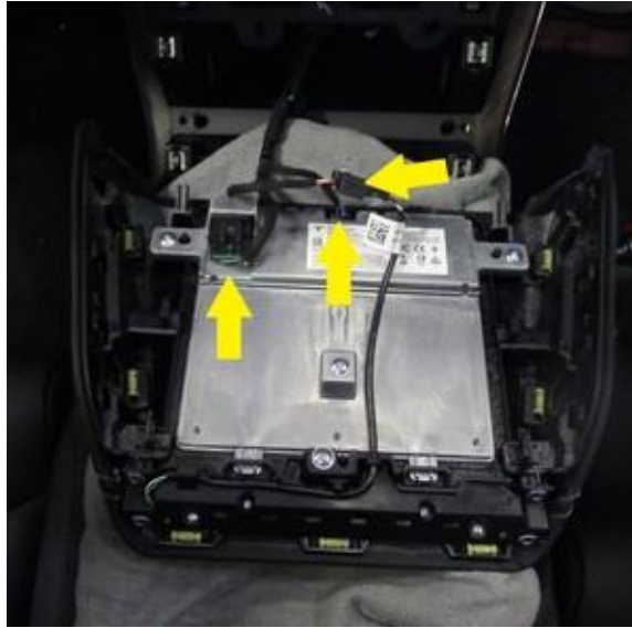
Figure 22. Releasing the phone dock connectors
