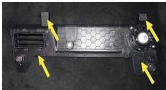
Figure 36. Releasing the RH footwell
