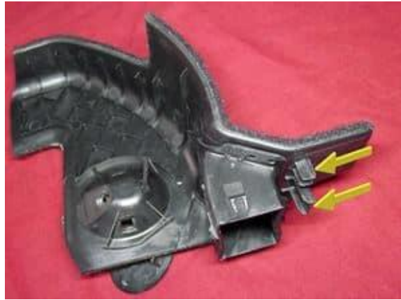
Figure 31. Releasing the LH inboard footwell
