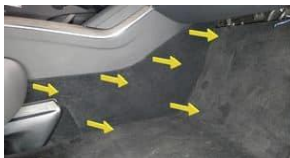
Figure 37. Releasing the RH console side carpet
