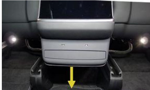
Figure 1. Detach the console
