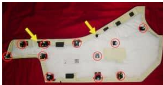
Figure 33. Releasing the LH console side carpet
