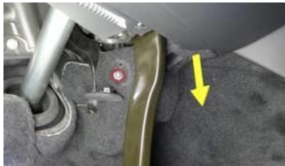
Figure 30. Releasing the LH inboard footwell
