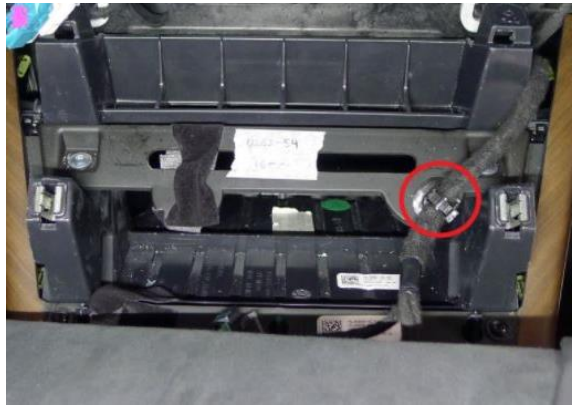
Figure 6. Releasing the phone dock wire clip
