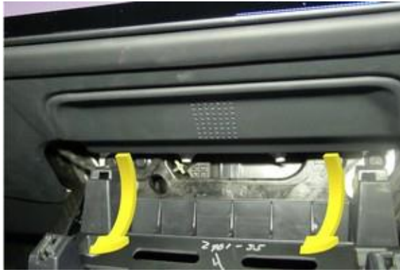
Figure 9. Removing the IP service panel
