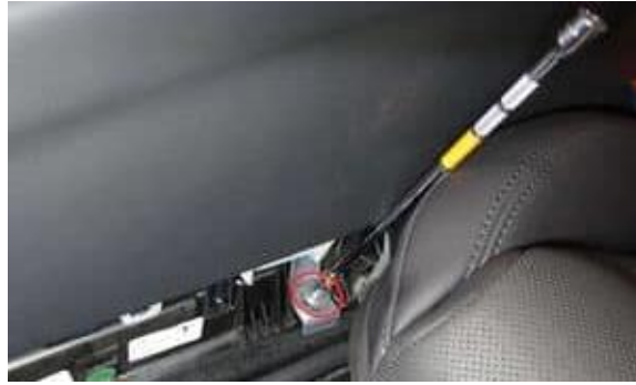
Figure 41. Releasing the console carrier center bracket (LH side)
