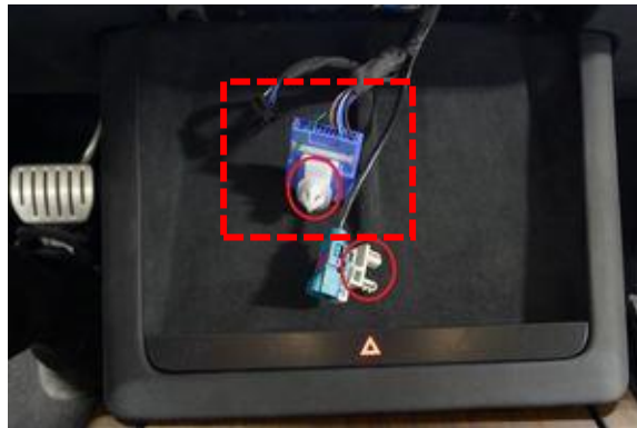
Figure 10. Moving the vehicle communication harness into position
