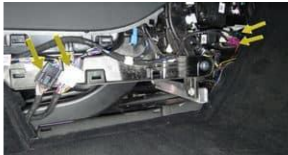
Figure 40. Releasing the center console connectors
