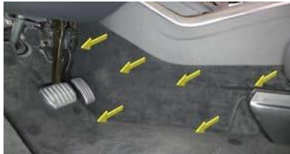
Figure 32. Releasing the LH console side carpet
