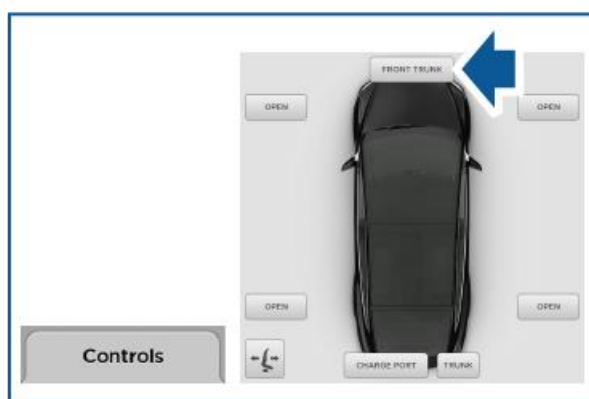
Figure 62. Opening the front trunk using the touchscreen
