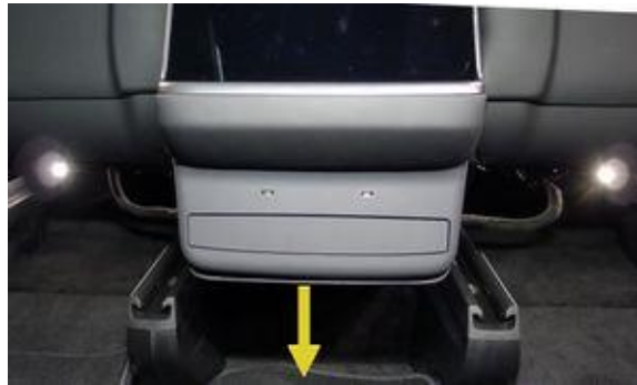
Figure 14. Detach the console
