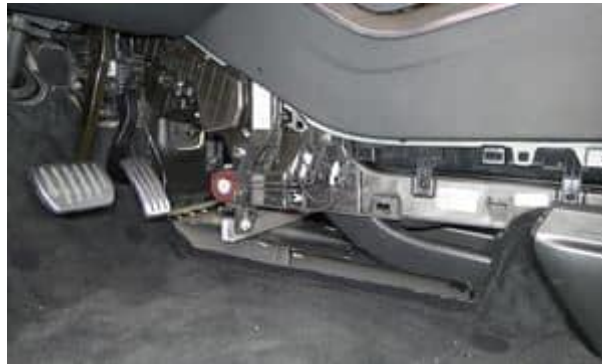
Figure 34. Releasing the LH center console lower bracket
