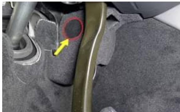
Figure 29. Releasing the LH inboard footwell
