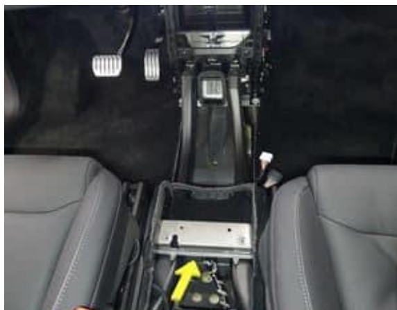
Figure 51. Disconnect the RCM connectors
