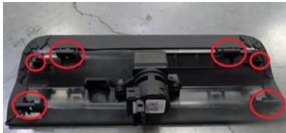
Figure 23. Removing the IP service panel
