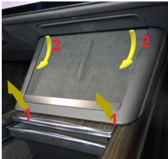
Figure 20. Releasing the phone dock
