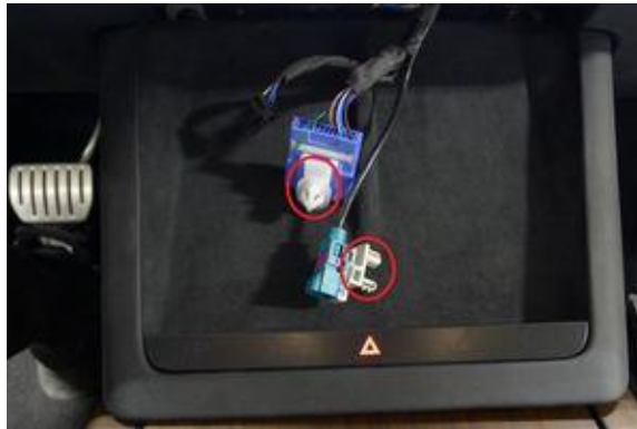
Figure 25. Releasing the diagnostic and CAN harnesses
