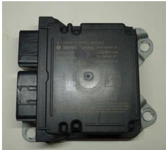
Figure 57. RCM removed from the vehicle
