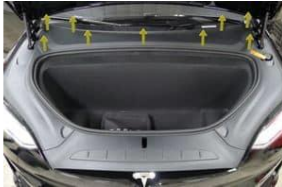
Figure 47. Removing the underhood apron
