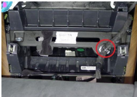
Figure 21. Releasing the phone dock wire clip
