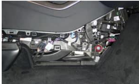
Figure 39. Releasing the RH center console lower bracket
