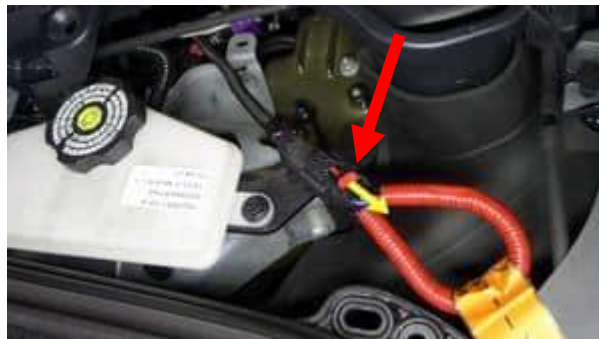
Figure 68. Disconnecting the first responder loop harness
