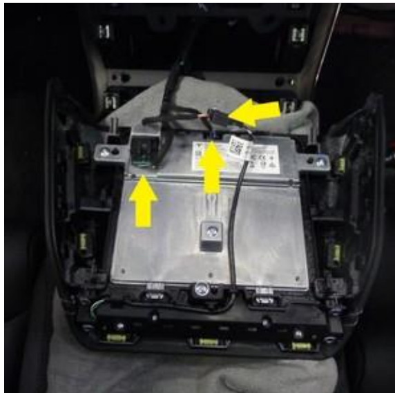
Figure 7. Releasing the phone dock connectors
