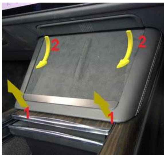
Figure 5. Releasing the phone dock
