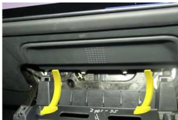
Figure 24. Removing the IP service panel
