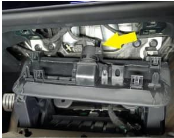
Figure 26. Releasing the IP service panel
