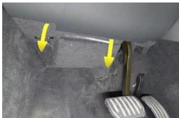
Figure 27. Releasing the LH outboard footwell
