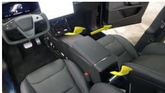
Figure 43. Releasing the LH console side carpet
