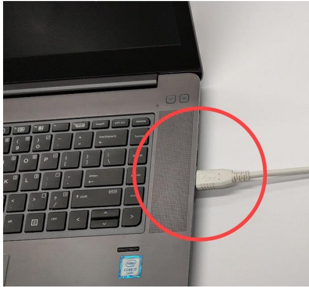
Figure 54. Connecting the PCAN to the computer
