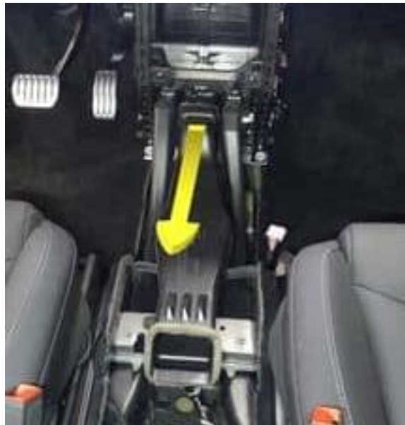
Figure 45. Center console HVAC duct
