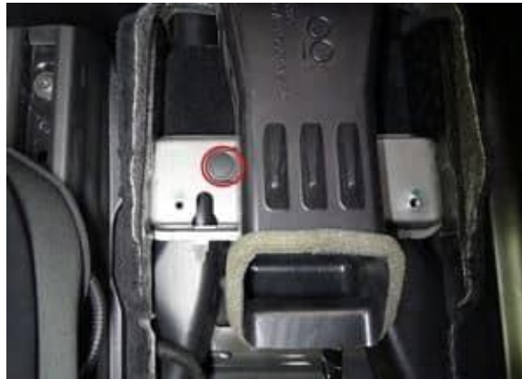
Figure 44. Center console HVAC duct
